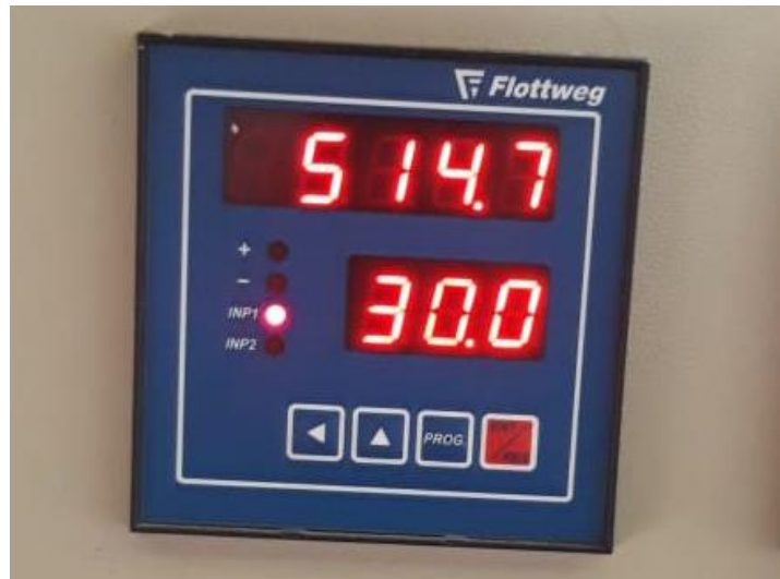
Gambar 14 Speed Test Putaran Motor Scroll, Scroll dan Bowl Speed
