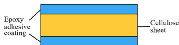
Fig. 1. Schematic illustration of epoxy adhesive resin coating arrangement on the cellulose sheet surface.
