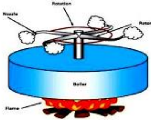
Gambar 3. 5 Prinsip Turbin Reaksi
